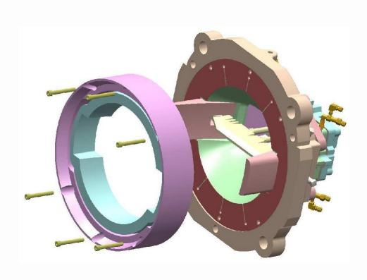
Bolts should be torqued to 250 ft/lbs on dies attached to J.C. Steele 90 machines.
