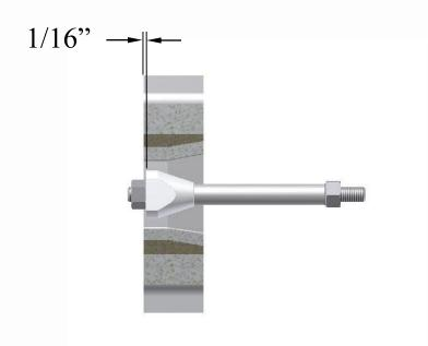
• All Die Combinations are figured so that the Cores are recessed 1/16" (1.5875 mm) inside the Face of the Cap
